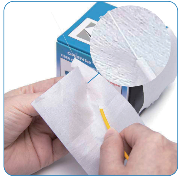
Direct wiping of bare optical fibers
