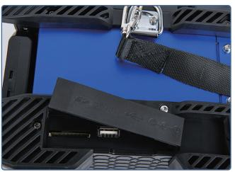
TERMINAL USB,SD,External Power.Silica gel pads are more effective in protecting machines.
