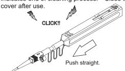
Be careful not to slant SC connector while inserting into the Guide cap.
