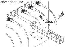
Be careful not to slant the Cleaner SC while inserting into the adapter.
