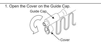
2. Insert SC connector into the Guide Cap.
